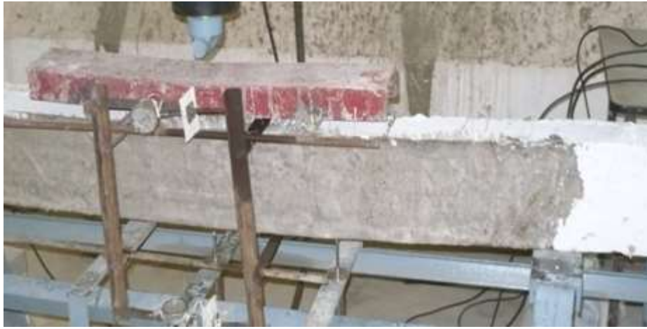
Fig 8. Arrangement Strain Measurement and LVDT-Deflection
