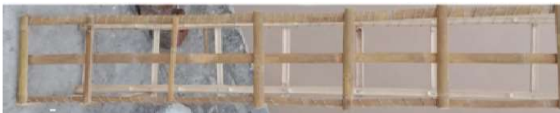
Fig 2 Model 2 (M2) Bamboo straps 20mmX10mm average size of 4 at bottom and 3 at top
