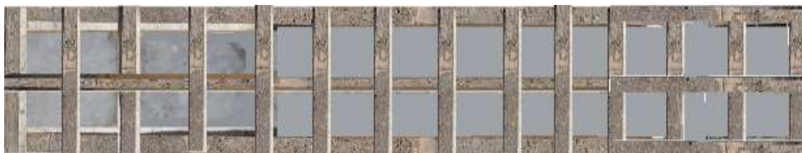
Fig 4 Model 3 (M3) straps are coated resin and sprayed with M-Sand 20mmX10mm
