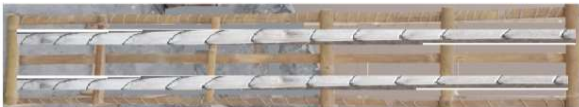
Fig 3 Model (M4) has 2mm binding wire with 20mm spacing spiral and coated with synthetic resin
