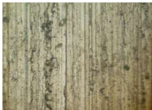
FIGURE 3 POLYMETALLIC MELT MICROSTRUCTURE (RESOLUTION 500X)
