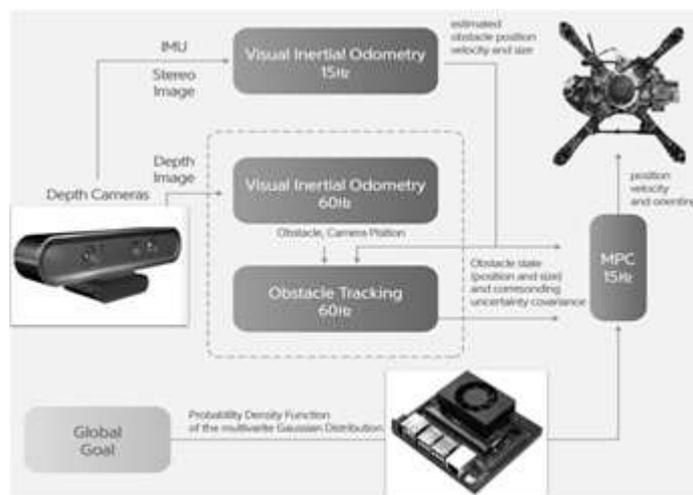
**Fig. 1:** System Hardware Configuration
