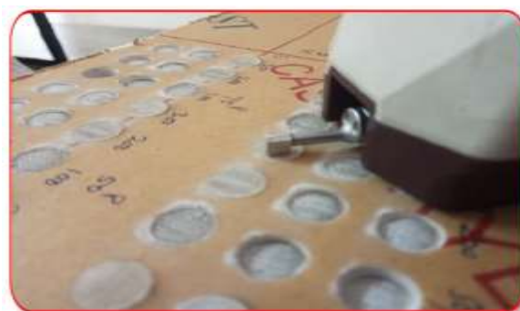
Figure 5 Surface roughness measurement process
