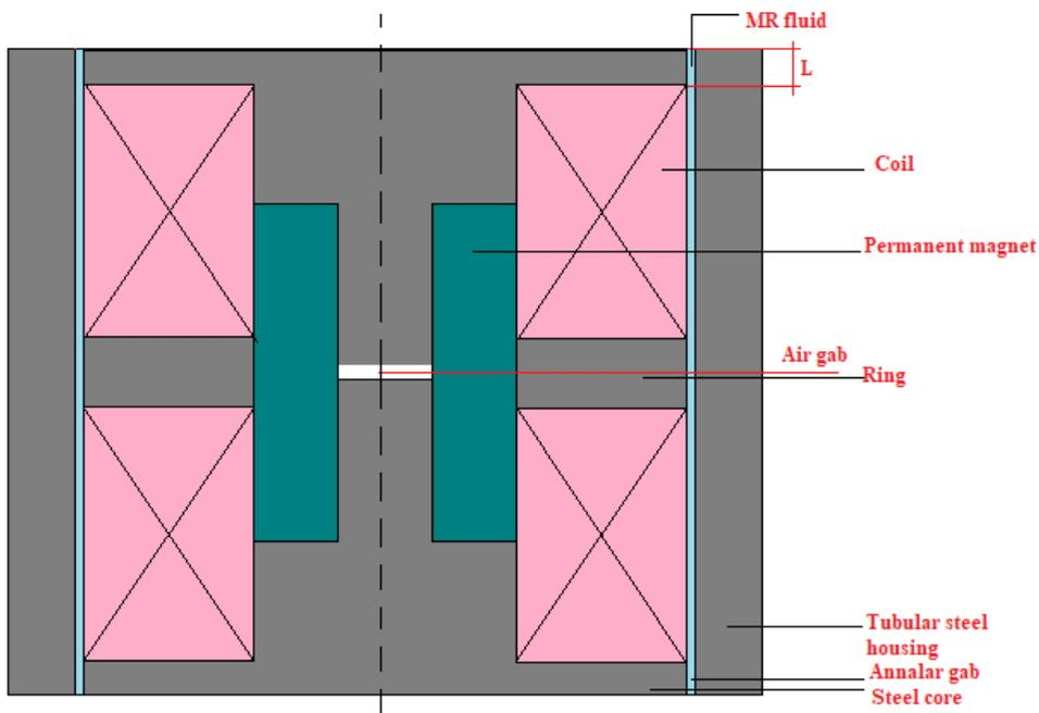
(a) The schematic of double coil NC MR valve with an annular gap.
