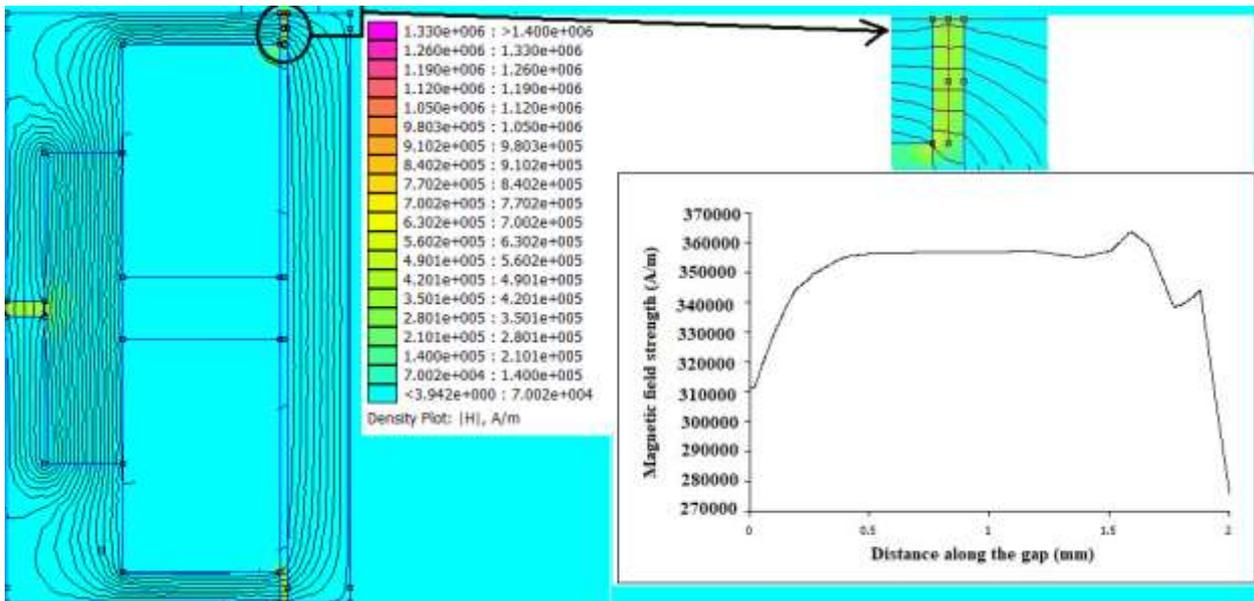
Figure 9: The annular NC MR valve magnetic field strength (H) result.
