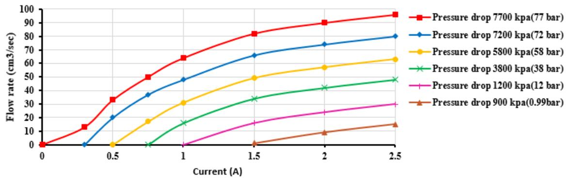
Figure 14: Reasonable relation between current and flow rate and pressure drops.
