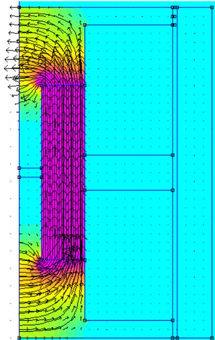
**Figure 7: The double coil NC MR valve magnetic flux direction.**
