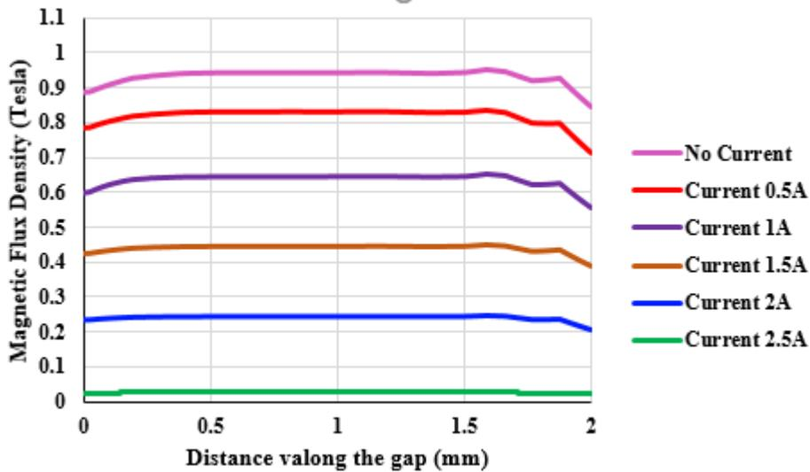
Figure 10: The magnetic density (B) along the annular NC MR valve gap.
