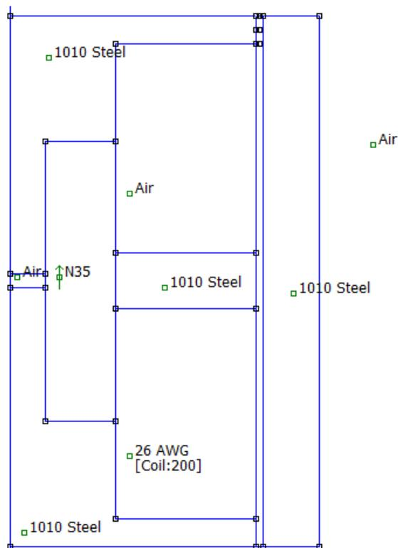
Figure 5: The FEMM dimensions of twin coil NC MR valve.
