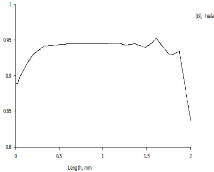
Figure 12: The FEMM software of the annular NC MR valve when  $I=0A$ .
