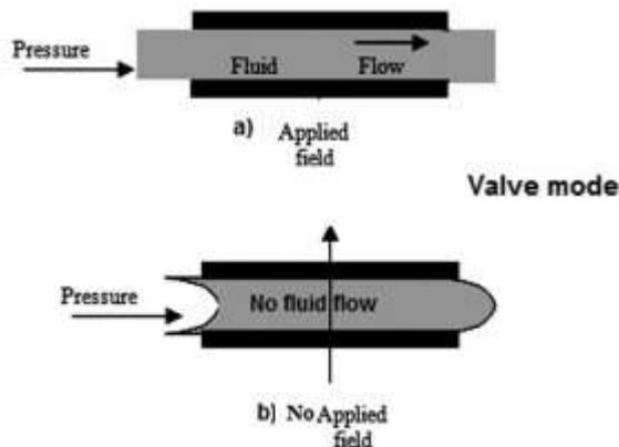
Figure 3: This diagram depicted the mode of Pressure of NC MR double coil fluid flow.
