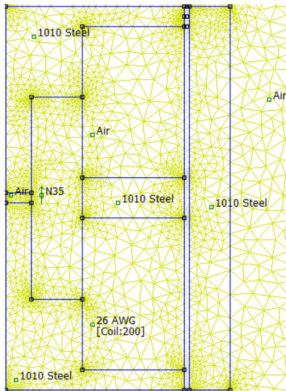
Figure 6: The model of twin coil NC MR valve in FEMM software.
