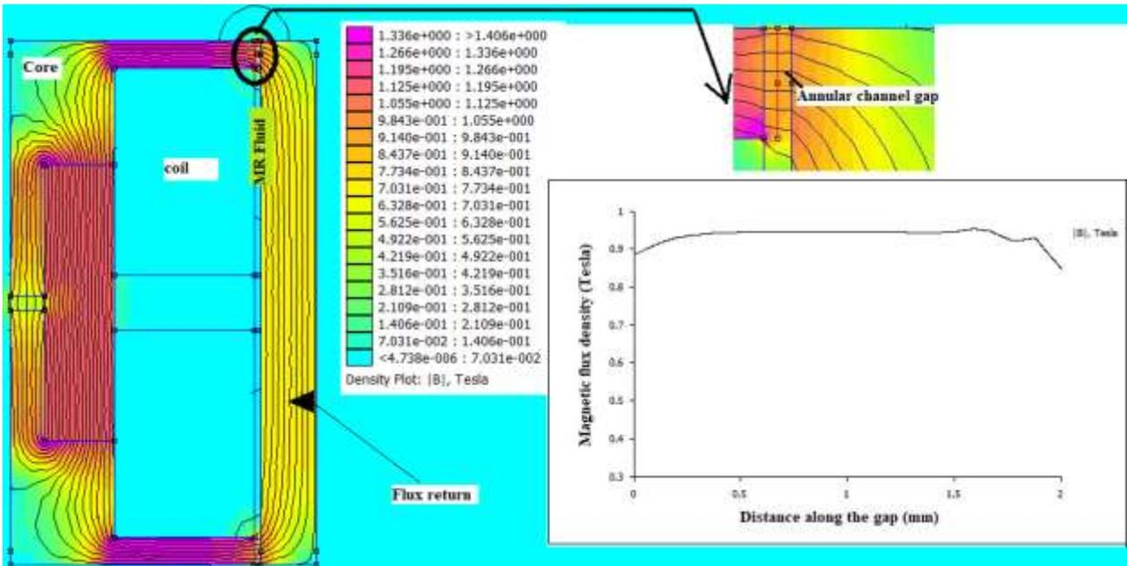
Figure 8: The annular NC MR valve flux density(B) result.
