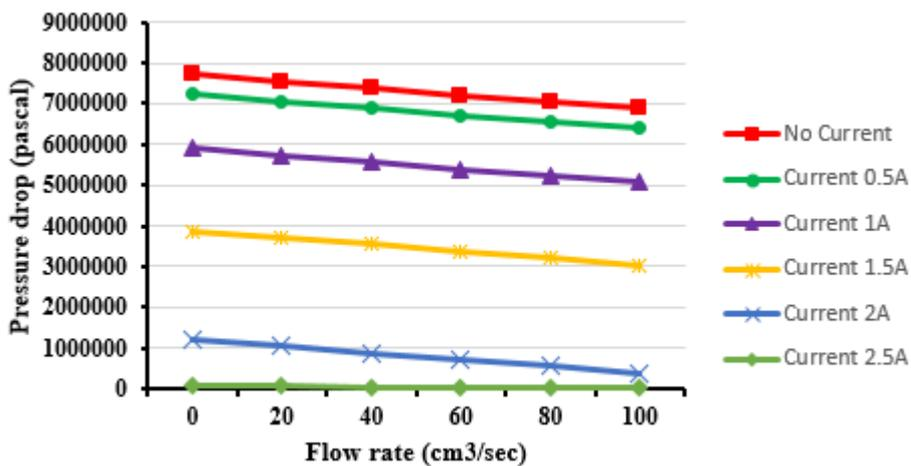
Figure 11: Relation between flow rate (Q) and pressure drop for different currents in annular NC MR valve.
