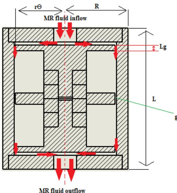
Figure 4: Modeling of the NC MR valve using annular flow paths plus double coil
