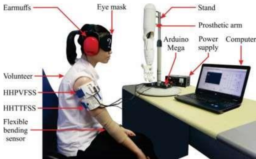
Figure 8: Set-up for the experiment: determining the effectiveness of the haptic wearable device in conveying tactile information.
