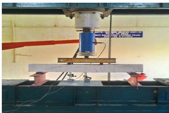
Fig.4: Test setup for flexural behavior of RC beam
