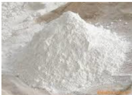
Fig. 1: Physical Appearance of Metakaolin
