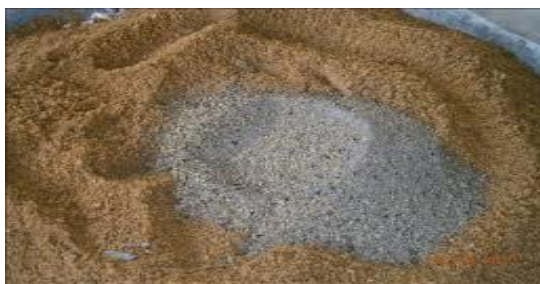
Fig. 2: Physical Appearance of Bottom Ash
