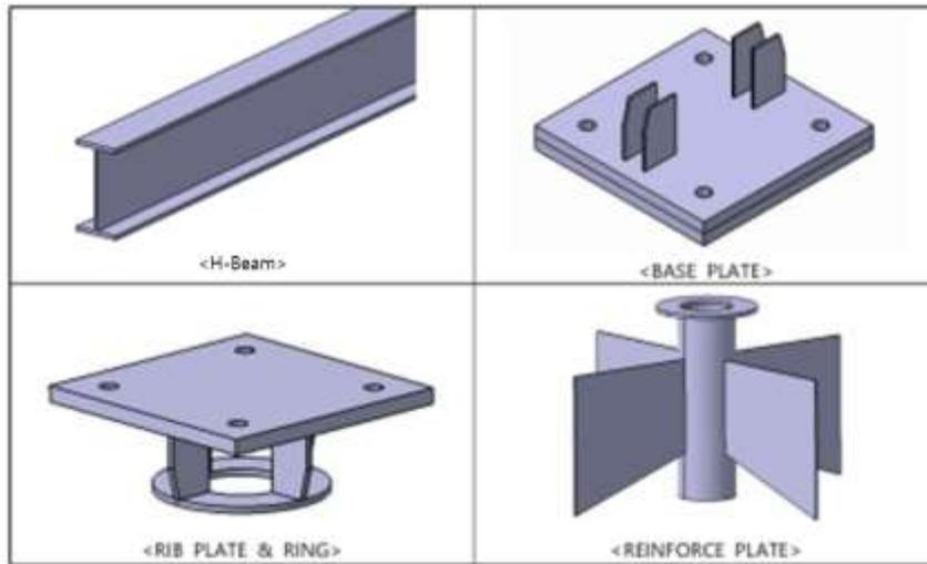
Fig. 2 3-D modeling of screw parts
