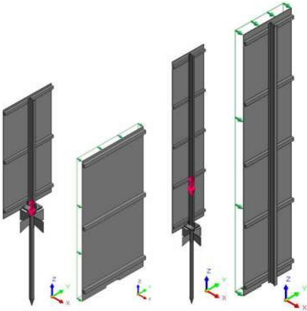
Fig. 6. Wind pressure and gravity loading conditions
