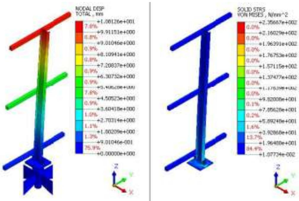
Fig. 10 Displacement and stress distribution of bolted structure (3mX3m)
