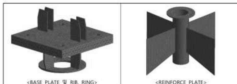
Fig. 4 3-D modeling of base plate and reinforcement plate
