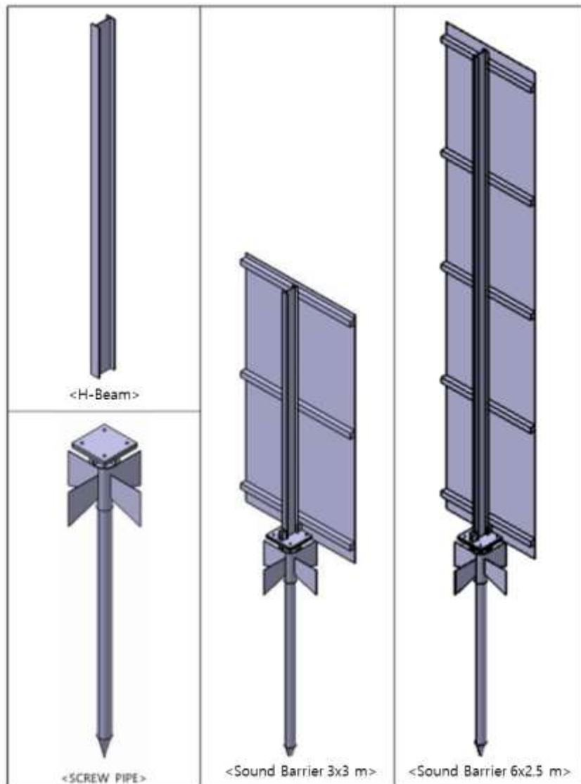
Fig. 3-D modeling of H-beam steel, screw pile and sound barrier assembly
