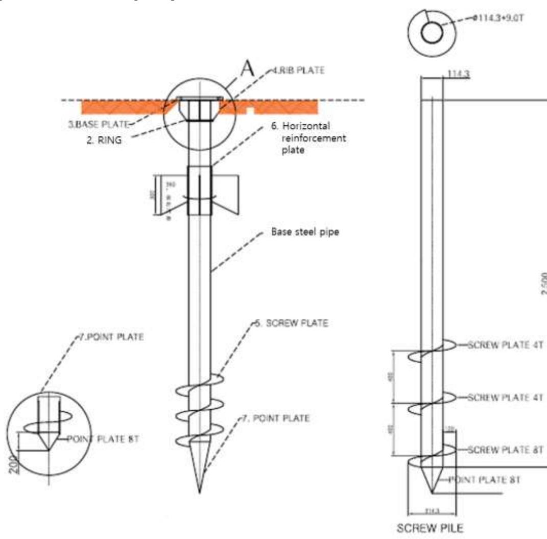
Fig. 1 Manufacturing drawing for screw pile
