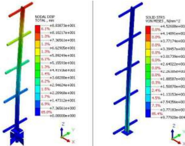
Fig. 9 Integral structure (6mX2.5m) displacement and stress distribution
