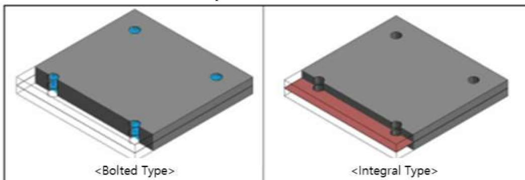
Fig. 7. Contact conditions of base plate top and bottom
