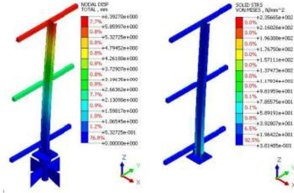
Fig. 8 Integral type structure (3X3m) displacement and stress distribution diagram
