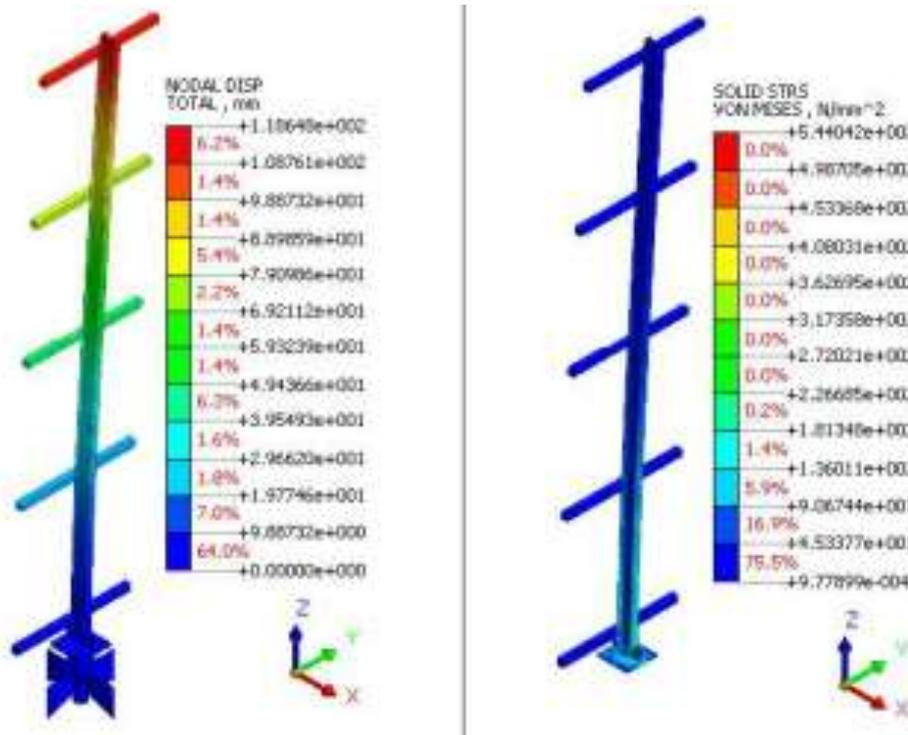
Fig. 11 Displacement and stress distribution of bolted structure (6mX2.5m)
