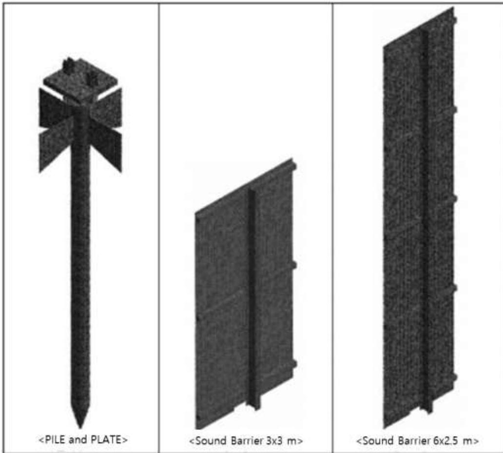
Fig. 5 3-D modeling assembling pile plate, H-beam and sound barrier
