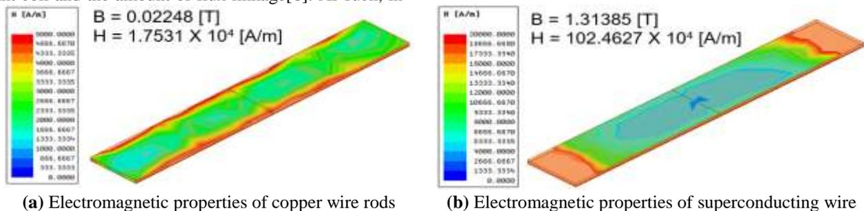
Figure 1. Electromagnetic properties of wire rods according to material
