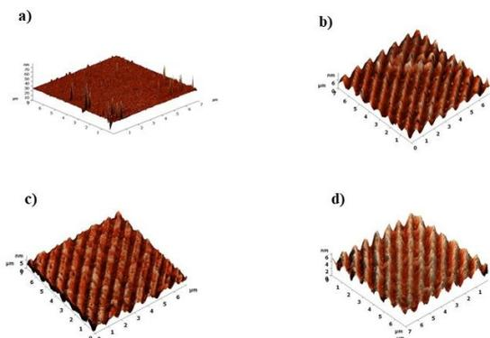
**Figure 1.** Representative image of glass cover slip control (a), coverslip scratched with silicon carbide paper p80 (b), p600 (c) and p1000 (d). The scanned area is 7x7 sq.μm.
