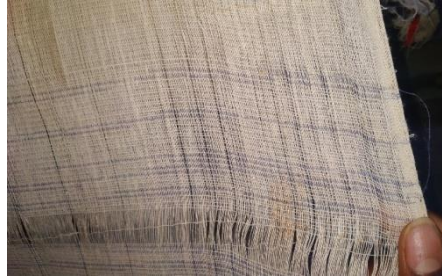
Fig.2.2-Trial fabric with no Weft holding mechanism
