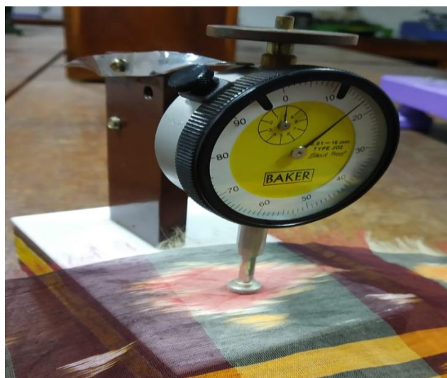
Fig.3.3- Fabric Thickness Tester
