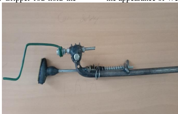
Fig.2.1-Appearance of Weft holding mechanism
