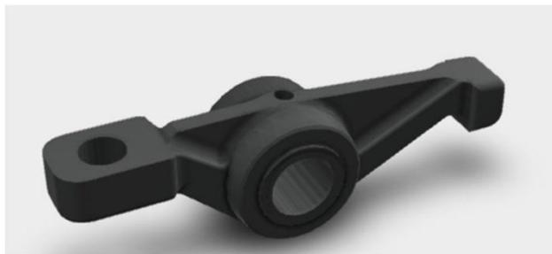
**Figure 2 Cad model of Rocker Arm**
