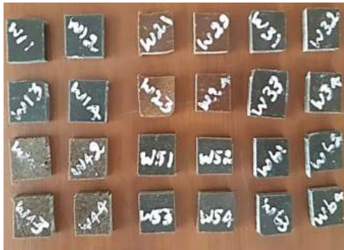
Figure 3 Water absorption test specimens after test
