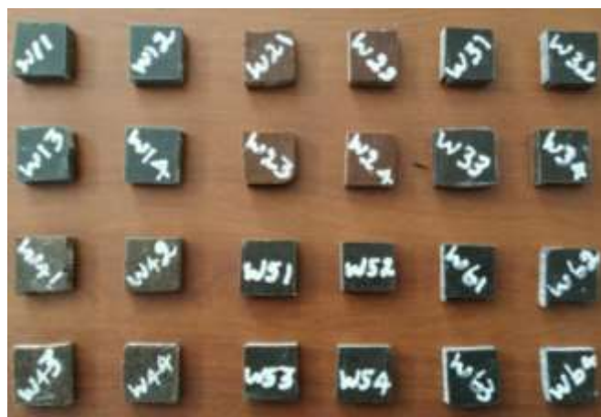
Figure 2 Water absorption test specimens before test
