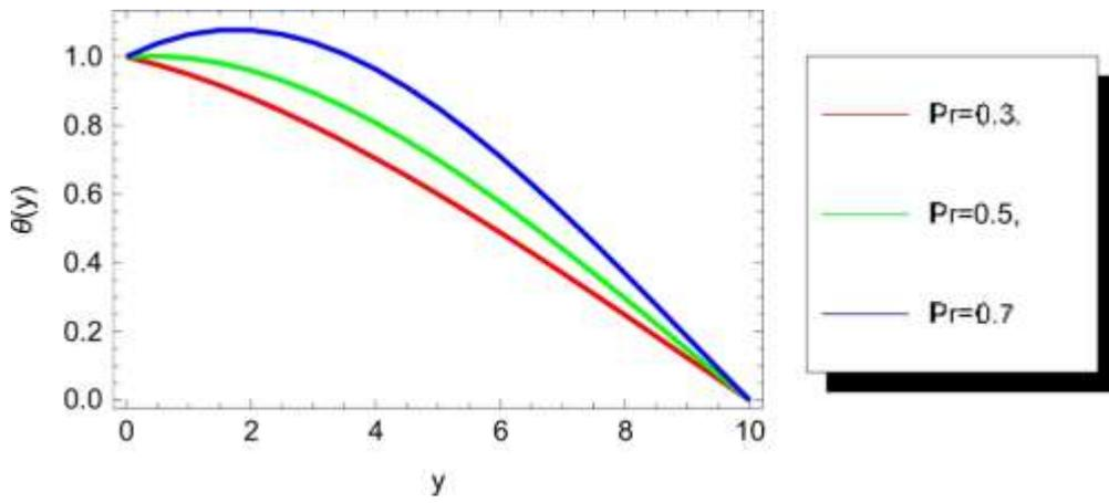
Figure 6: Variation of  $Pr$  on rate of heat transfer
