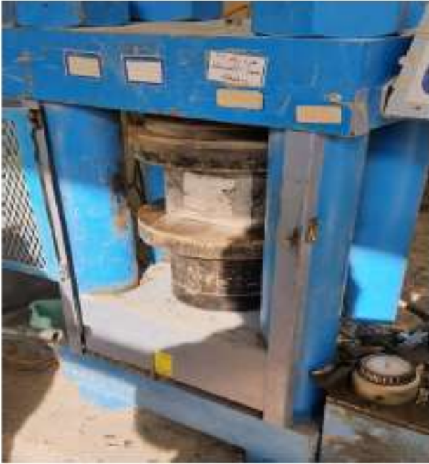
Plate (5): Compressive Strength Test
