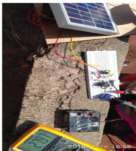
Figure 17 (B). Boost converter circuit input given by solar panel Output
