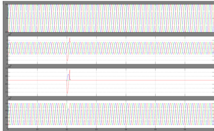
Figure7: Voltage sag (LLG Fault) (a) voltage of grid (b) voltage of load (c) compensated voltage (d) PCC voltage
