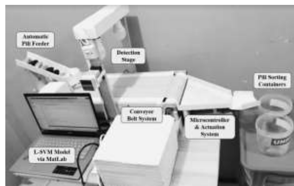
Fig. 4 Prototype of the Automated Pili Fruit Sorting Device.
