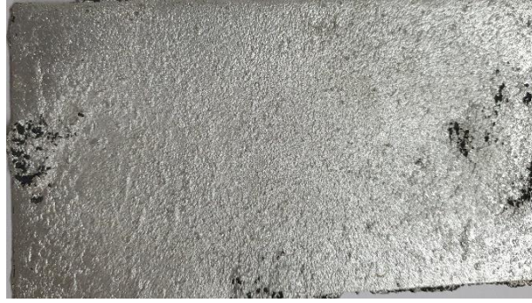
Fig 2 : Al7075 MMC sheet of 10mm thickness
