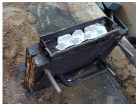
Fig 4. MMC plate produced after stir casting
