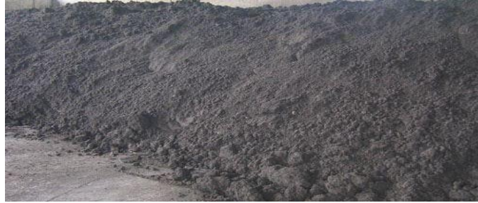
Figure 2. Sample image of dry sludge.
