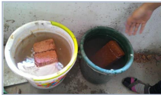
Figure 8. Absorption of water by bricks.
