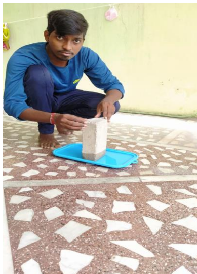
Figure 8: Performing efflorescence test at home
