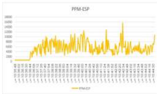
figure (13) CO 2 level inside the mask by ESP-32
