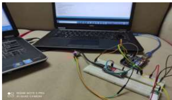
Figure (4) MQ-135 Sensor connects with Arduino Uno and ESP-32
