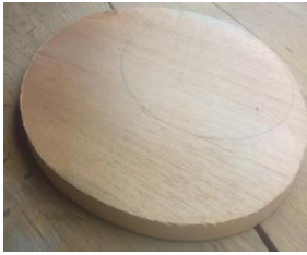
Figure 25: Wood slab support for chasing
