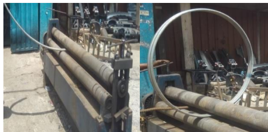
Figure 39: Bending of galvanized pipes on a bending mill
