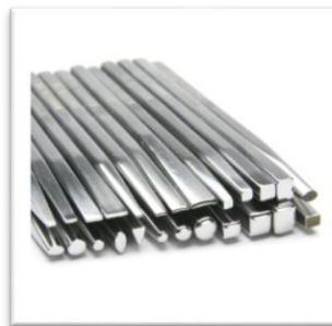
Figure 5: Chasing and repousse tools
