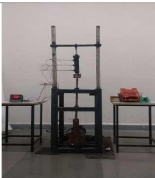
Figure 1: Experimental Set-up for Shock Absorber
