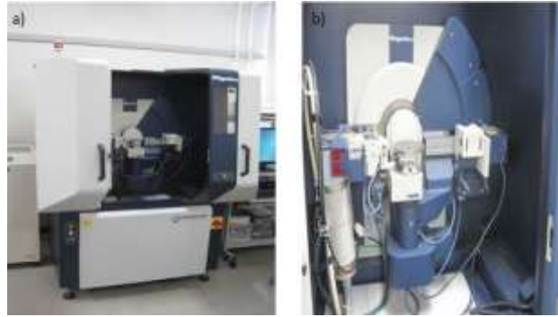
Fig. 8: XRD instrument a) Setup of XRD b) Place for holding the slide during the XRD.
