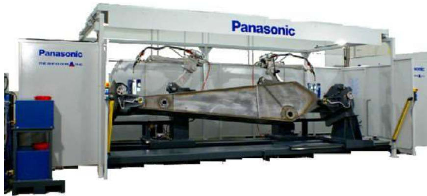
Fig 3 Panasonic Perform Arc robot
