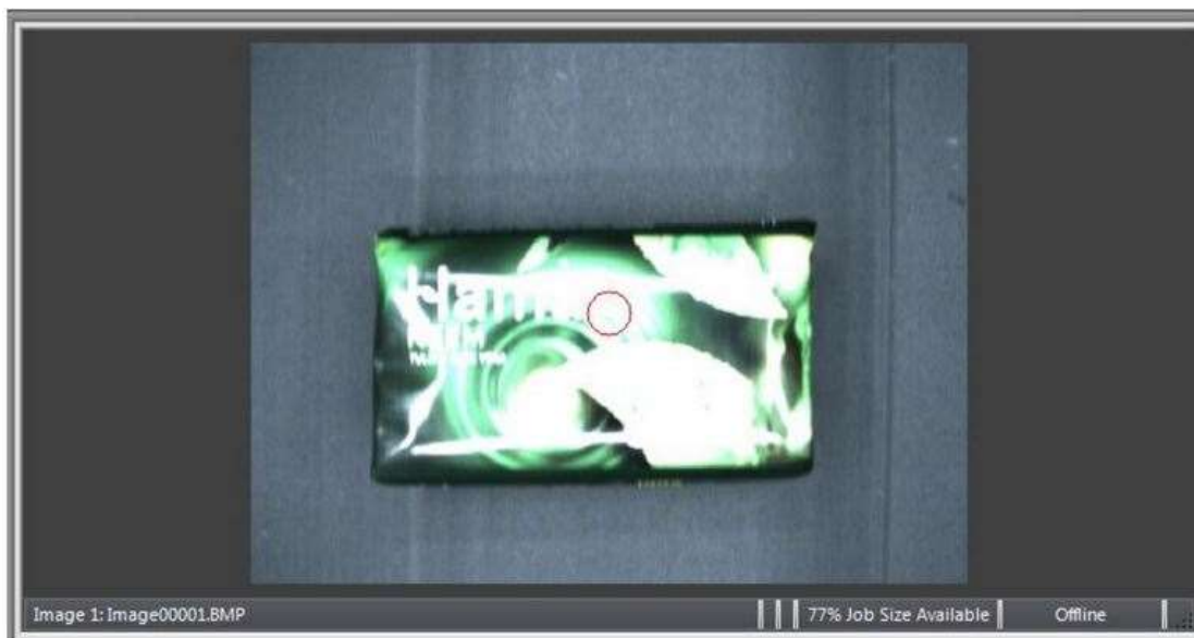
Figure Camera Inspected Product in HMI Display
