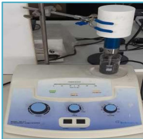
**Figure (2): Ultrasound Mixing Device.**
