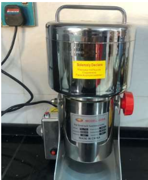
Figure 3. High Speed Multi-Functional Crusher
