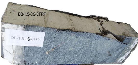
Figure (11): Failure mode for Rehabilitation Deep Beam with (a/d=1.5) failed in shear - DB-1.5-CS-CFRP
