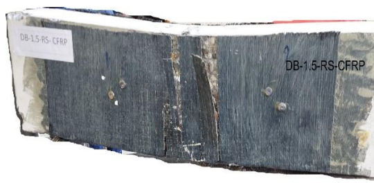
Figure (12): Failure mode for Rehabilitated Deep Beam with (a/d=1.5) failed in shear - DB-1.5-RS-CFRP
