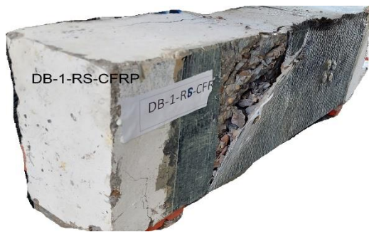
Figure (10): Failure mode for Rehabilitated Deep Beam with (a/d=1) failed in shear - DB-1-RS-CFRP
