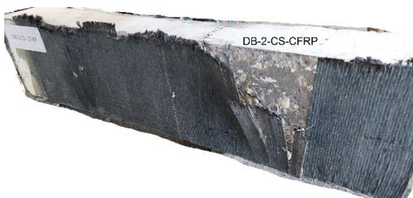
Figure (13): Failure mode for Rehabilitated Deep Beam with (a/d=2) failed in shear - DB-2-CS-CFRP
