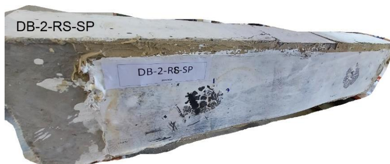
Figure (23): Failure mode for Rehabilitation Deep Beam with ( a/d=2 ) fail in shear - DB-2-RS-SP
