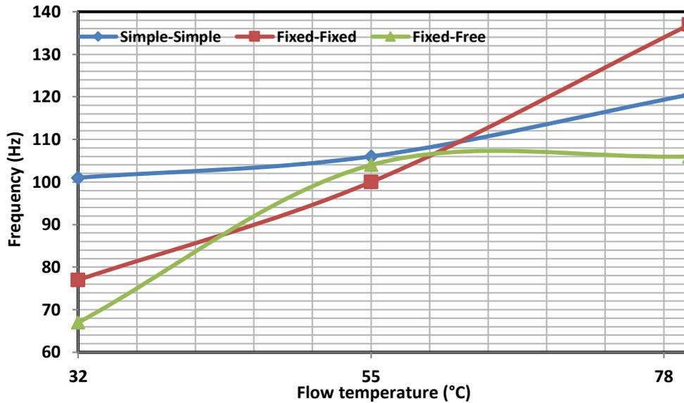
Figure 7. Variation of frequency with flow temperature in bellow at diameter 10 mm with flow rate 14 LPM
