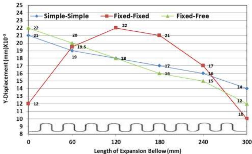
Figure 8. Variation of Y-displacement with the length of bellow at 20 mm diameter, 80 °C and 14 LPM
