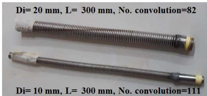
Figure 1. Types of expansion bellows
