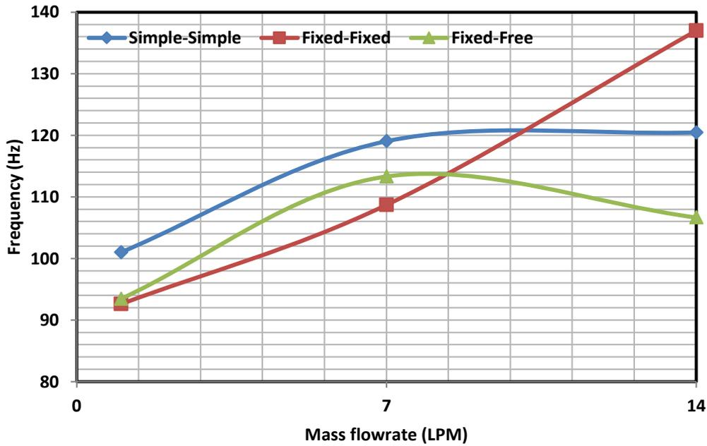
Figure 5. Variation of frequency with flow rate in bellow at diameter 10 mm in flow temperature 80 °C
