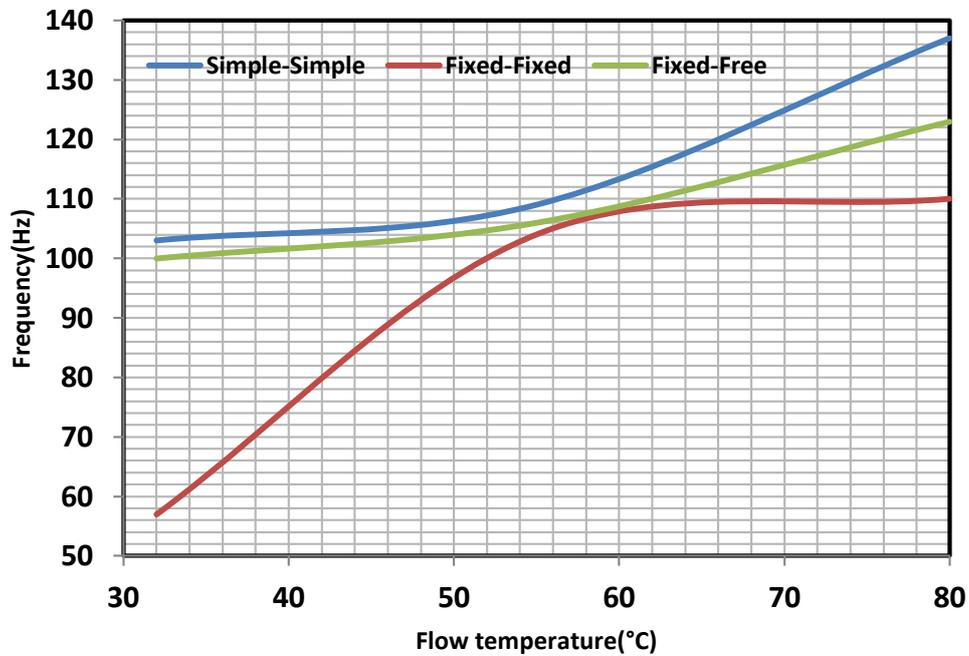
Figure 6. Variation of frequency with flow temperature in bellow at diameter 20 mm with flow rate 14 LPM
