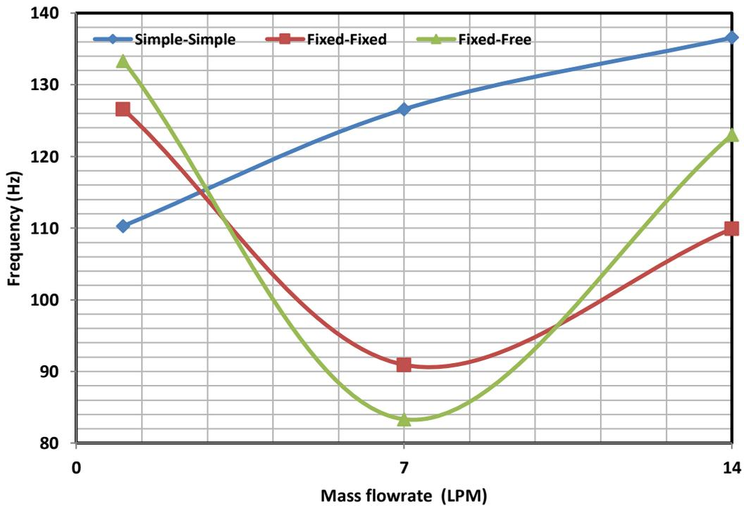
Figure 4. Variation of frequency with flow rate in bellow at diameter 20 mm in flow temperature 80 °C
