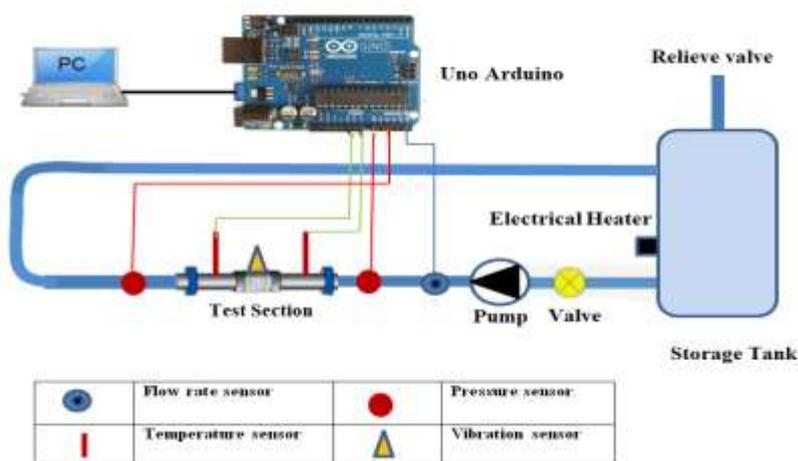
Figure 3. Schematic diagram of system
