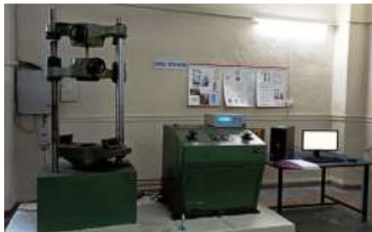
Fig.7 Universal Tensile Testing Machine used for tensile and flexural test
