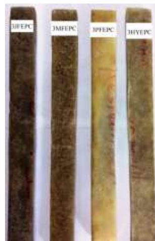
Fig 6. Composite samples prepared by hand lay up process
