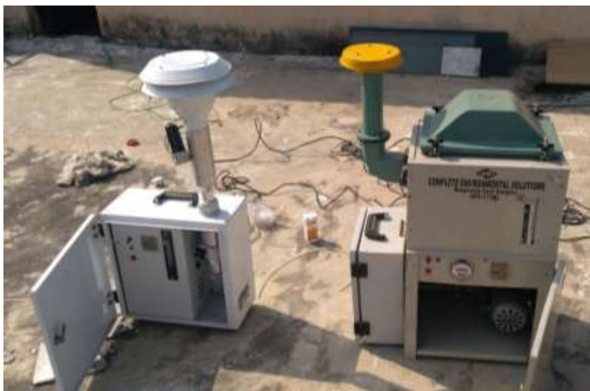
Fig. 2 Respirable Dust Sampler used for sample collection
