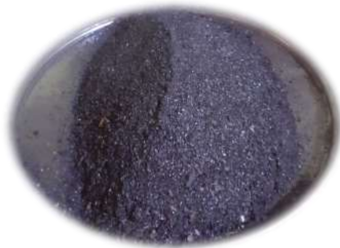
Fig. 1: Sample of the iron fillings waste used in the study.
