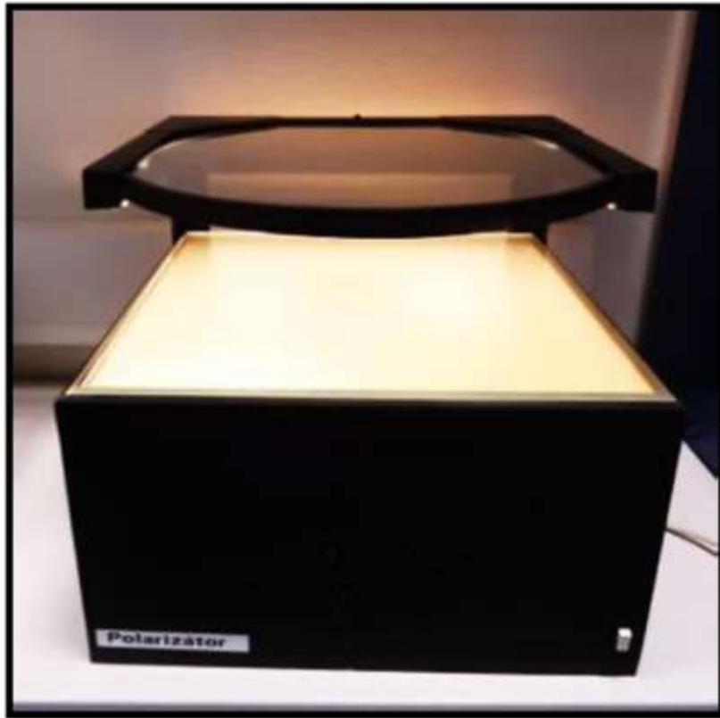
Figure (4): Polariscope with light source and polarizer [4]
