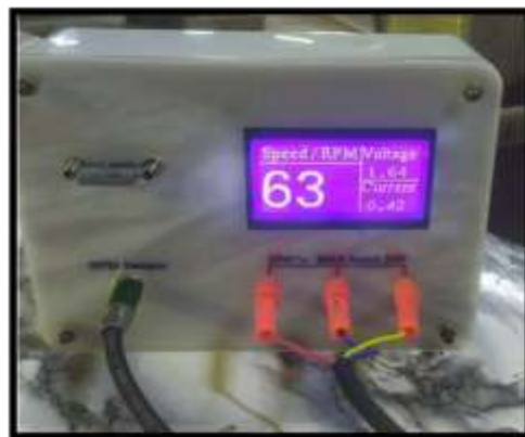
Fig. (4). A device (three in one) for measuring rotational speed, voltage and current
