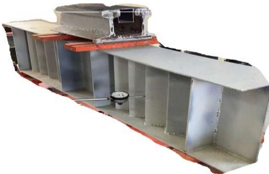
Figure 4: Preparation of Plate Girder.
