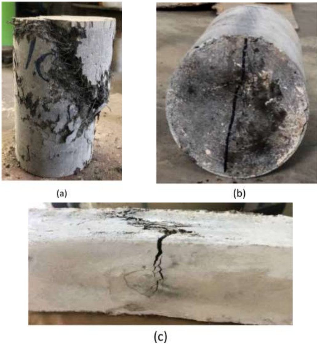
Figure 2: Failure patterns of cylinders and prisms. a) compressive fracture pattern, b) splitting tensile fracture pattern, c) prism failure pattern
