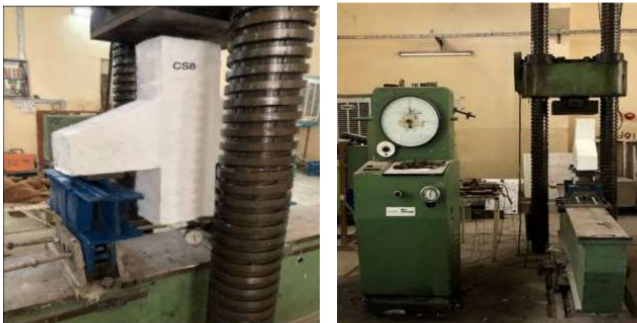
(a) (b) Figure 3: Test set up. a) Set up of corbel specimen, b) Testing machine
