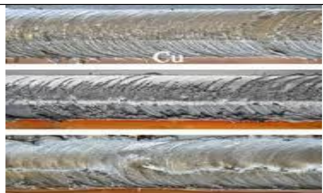
Fig:14 Defect are formed at high RPM due to this void and cracks are formed and we have compared it with micro structural images
