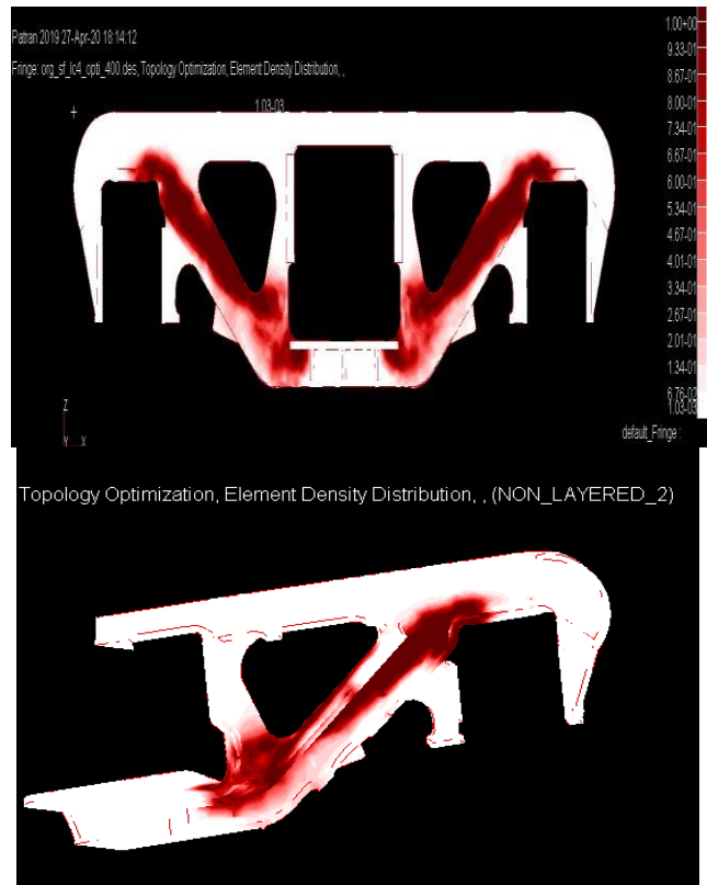
Fig. 4(a,b) : Topology optimized design showing element density distribution (Front view)
