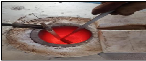
Figure 1: Formation of Al-Zn alloy
