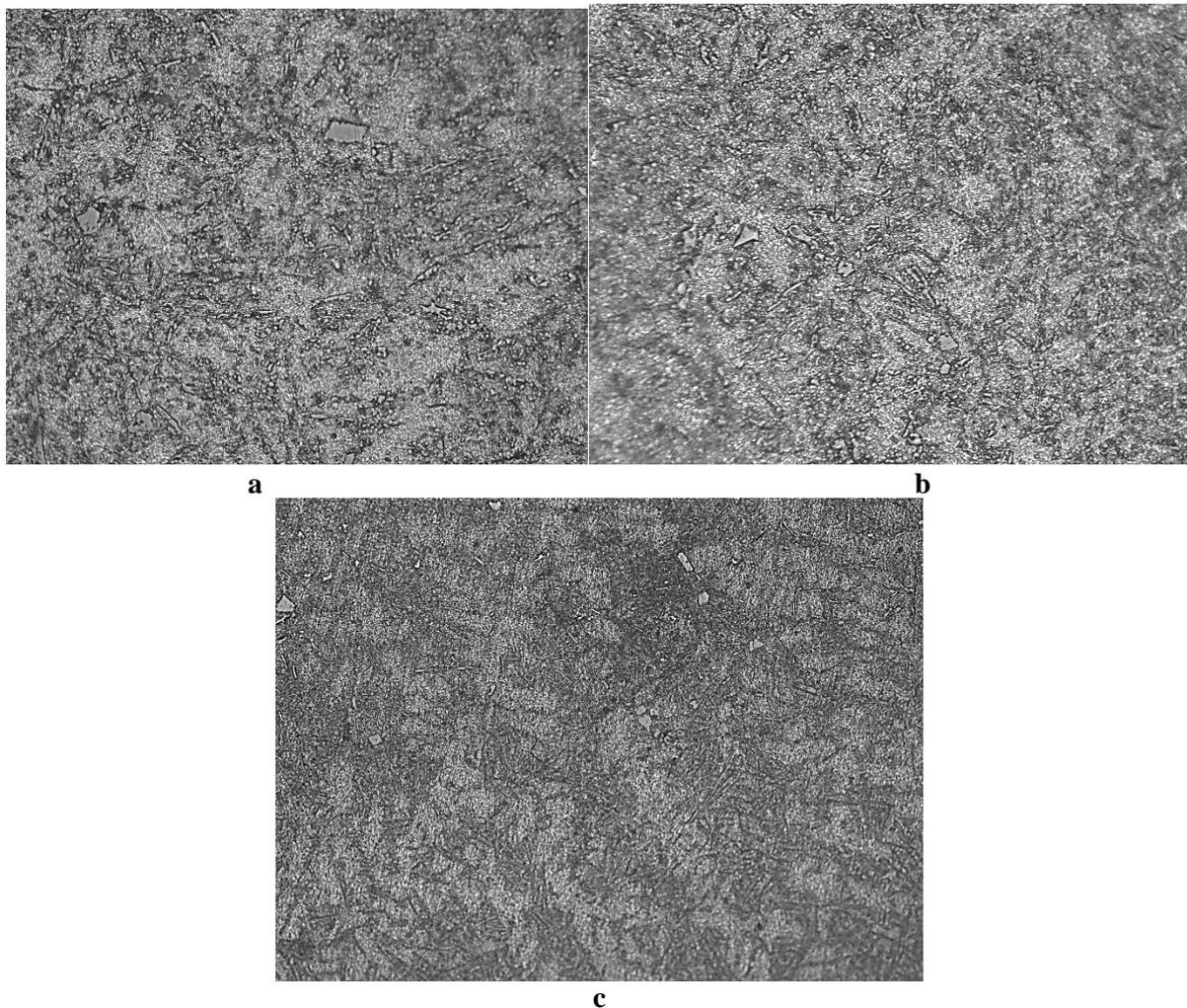
Fig. 2: Microscopic images (500X) Composite with (a) 2% Fly ash (b) 5% Fly ash (c) 8% Fly ash
