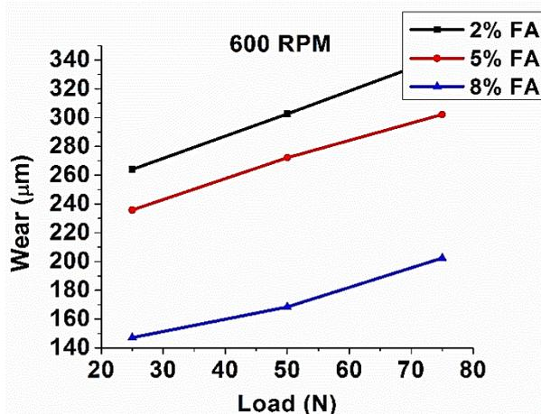
Fig. 8: Wear rate at different loads
