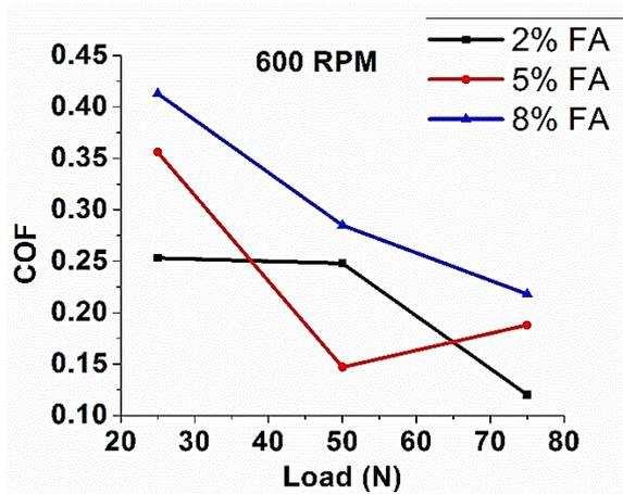
Fig.6: COF at different loads
