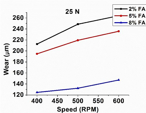
Fig. 9: Wear rate at different speeds
