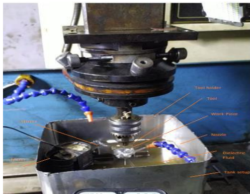
Figure 3: Experimental setup with accessories for micro- EDM
