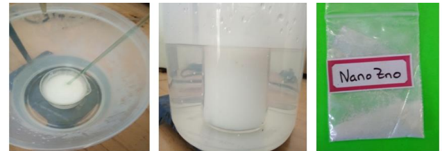
(a) Nano ZnOH (b) Nano ZnO Gel (c) Dried Nano ZnO Powder
