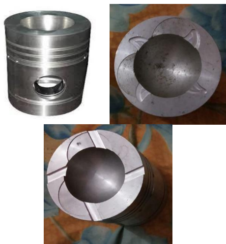
Figure 2.1 Image of Normal, Beak and Tangential Grooved Pistons Before Placing in to Cylinder
