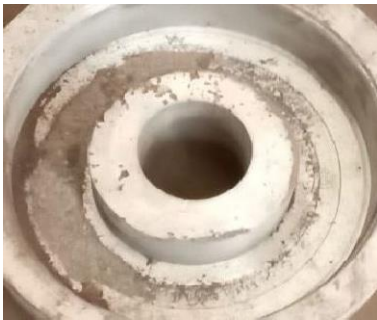
g. Erosion and mechanical sand sinters
