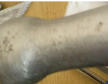
e. Pin holes and thermal sand sinters
