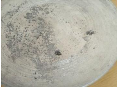
e. Pin holes and thermal sand sinters
