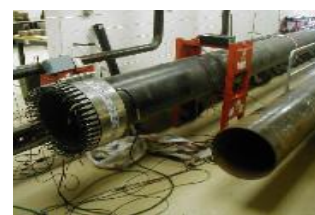
FIGURE 5 PHASED ARRAY FOCUSING PROBE. TELETTEST DEVICE, COURTESY OF I&T NARDONI INSTITUTE, BRESCIA – ITALY
