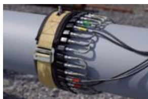
FIGURE 4 COMMERCIAL RING-SHAPE PROBE WITH PIEZOELECTRIC SENSORS
