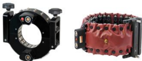
FIGURE 3 SOLID AND INFLATABLE COLLAR TYPE PROBES [5]
