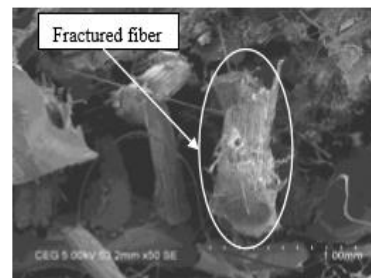
Fig. 3.4 “SEM micrographs of the “Hybrid “composite”” samples subjected to tensile loading”
