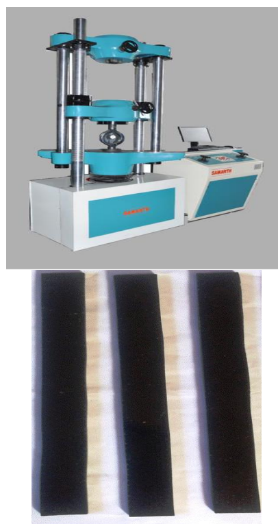
Fig. 2.6 Test set up for Tensile test and Specimens
