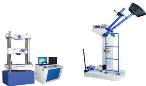
Fig. 2.6 Test set up for Tensile and Impact
