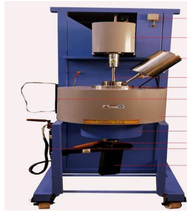
Fig.2. Bottom pouring stir casting equipment
